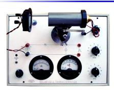
One panel mounted light source with variable intensity
