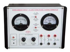
Two regulated DC supplies 0- 3V, and 0- 60 volts one germenium diode, two dual range meters, one for voltage and one for current. with range and mode select.
