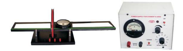
Current Carrying Coil Setup is useful to understand the concept of Electromagnetism. The product is also known as Stewart and Gee apparatus. This setup is helpful for the study of magnetic field around a current carrying coil. The setup illustrates how magnetic field generates by applying electric current in any current carrying conductor. For this purpose Tangent Galvanometer is used, which is based on Tangent law of magnetism.
